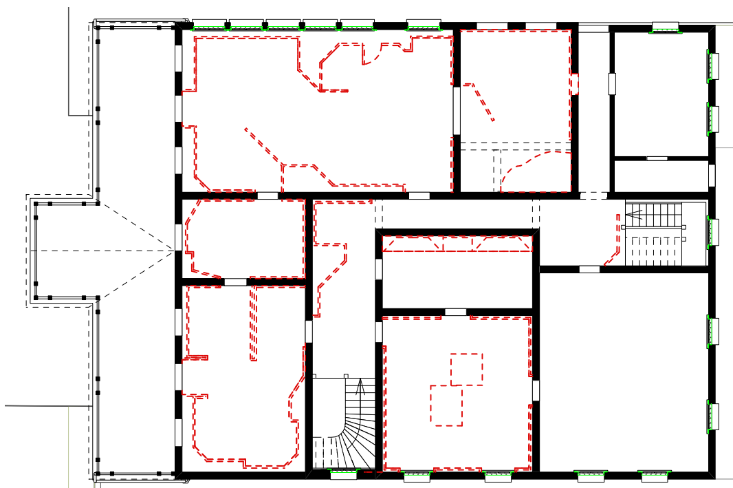
First Floor Demolition Plan
